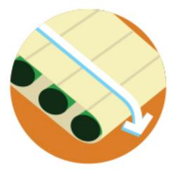
As recyclable material travels along the materials recovery facility (MRF) conveyor belt — a high-powered magnet attracts steel cans to separate them from other materials. The steel cans are then baled before shipment to a steel mill or foundry.
